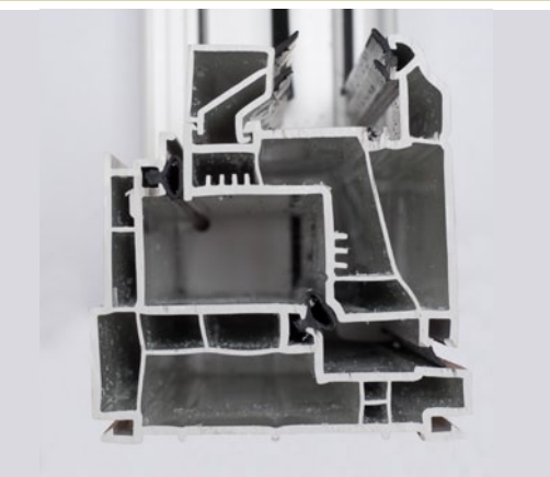
A cross section of a casement/awning window. Note the easily replaceable triple weatherstrips and high strength multichamber design.
